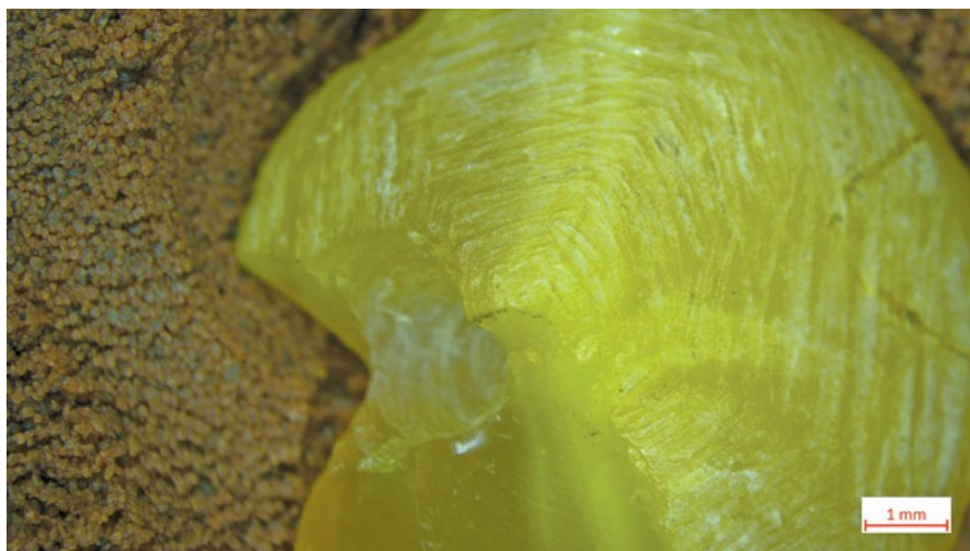
5. Damage that occurred during the perforation of the hole. An example from Šventoji 6, EM 2138:550, photo by Gvidas Slah
